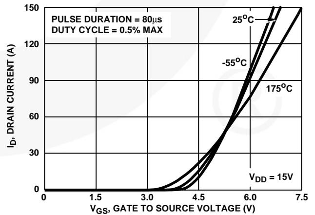
FIGURE 8. TRANSFER CHARACTERISTICS
