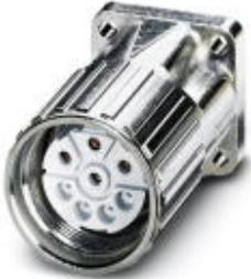
Device connector, front mounting with knurled nut, straight, Screw locking, M23, number of positions: 4+3+PE, type of contact: Socket, Crimp connection, Axial O-ring, 4x Ø 3.2, shielded: yes, flange dimensions: 26 mm x 26 mm, cable diameter range: 0 mm ... 0 mm
