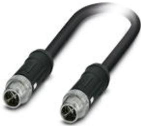
Network cable, Ethernet CAT6<sub>A</sub> (10 Gbps), 8-position, Elastomer electron beam cross-linked halogen-free, black, shielded, Plug straight M12 SPEEDCON / IP67, Coding: X, on Plug straight M12 SPEEDCON / IP67, Coding: X, Cable length: 5 m
