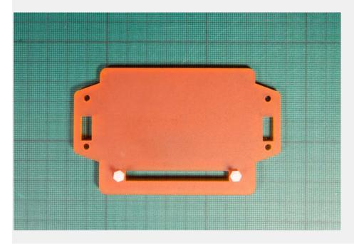
Push the two M2.5 bolts through the frosted orange layer and then screw two of the nuts on tight (these are the spacers). Now, slide your Scroll pHAT HD down onto the bolts, so that the LEDs are facing towards the acrylic. Use the remaining two nuts to secure the pHAT.
