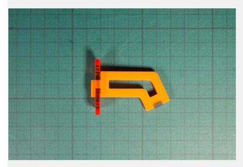
Place it into the recess on the back frosted orange layer, sliding it down over the two bolts. Do the same with the other leg, and then secure both with the M3 nuts.
