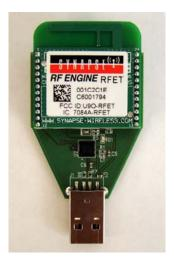
The Synapse SN132 SNAPstick USB module does not provide access to the entire range of GPIO pins available through the SN171 Proto Board. Instead, it provides a simple and compact way to connect a PC running Portal to a SNAP network.
