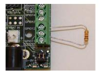
**Place** the other leg into the connector at GPIO 11. There is no polarity on this resistor, so it does not matter which leg you choose for which pin.
