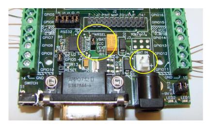
The board comes from the factory with the jumper connected to the VEXT and VCC pins, which configures the node to run from the external power supply.
