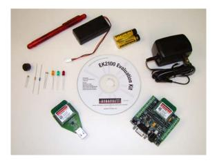
The EK2100 evaluation kit comes with management software, a power supply, an external battery holder, a pair of AA batteries, a screwdriver and a bag of components (refer to the *EK2100 Kit Contents* document). The kit also contains *two different kinds* of SNAP demonstration nodes:
