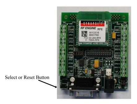
The Synapse SN171 Proto (prototyping) Board provides easy access to all 19 General Purpose Input/Output (GPIO) pins available on the SNAP RF Engine. 8 of these pins (GPIO 11-18) can also serve as analog inputs.
