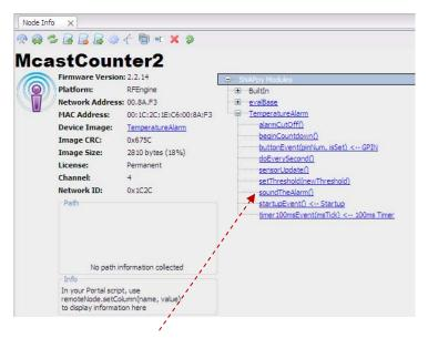
**Click** on the *soundAlarm()* function to test the buzzer. You should hear a long beep from the buzzer.
