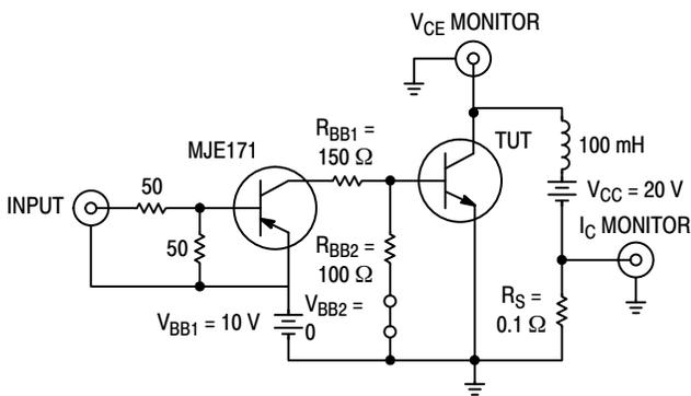
Note A: Input pulse width is increased until  $I_{CM} = 0.63\text{ A}$ .
