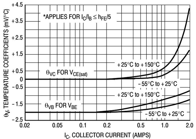
**Figure 7. Temperature Coefficients**
