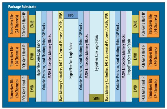
HPS: Quad ARM Cortex-A53 Hard Processor System
