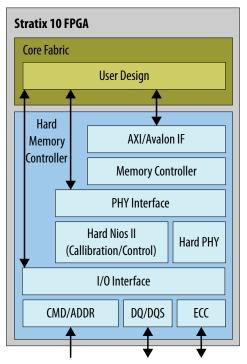
Each I/O bank contains 48 general purpose I/Os and a high-efficiency hard memory controller capable of supporting many different memory types, each with different performance capabilities. The hard memory controller is also capable of being bypassed and replaced by a soft controller implemented in the user logic. The I/Os each have a hardened double data rate (DDR) read/write path (PHY) capable of performing key memory interface functionality such as:
