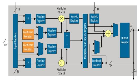
Figure 11. DSP Block: High Precision Fixed Point Mode
