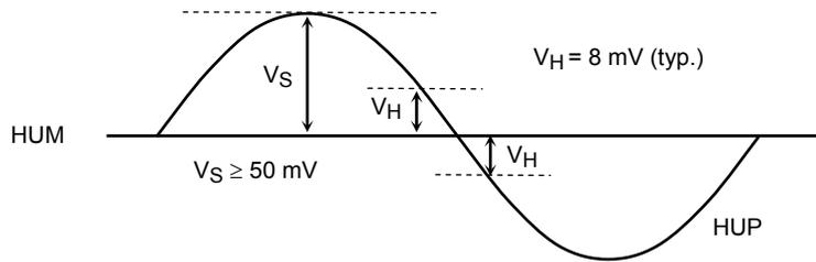
\*: The Hall amplifier can operate when V<sub>S</sub> is at least 50mVpp. However, to stabilize the time interval between zero-cross points of each phase signal, that is, the 60-electrical-degree interval, the amplitude should be as high as possible. (V<sub>S</sub> is recommended to be 200 mVpp or higher.)
