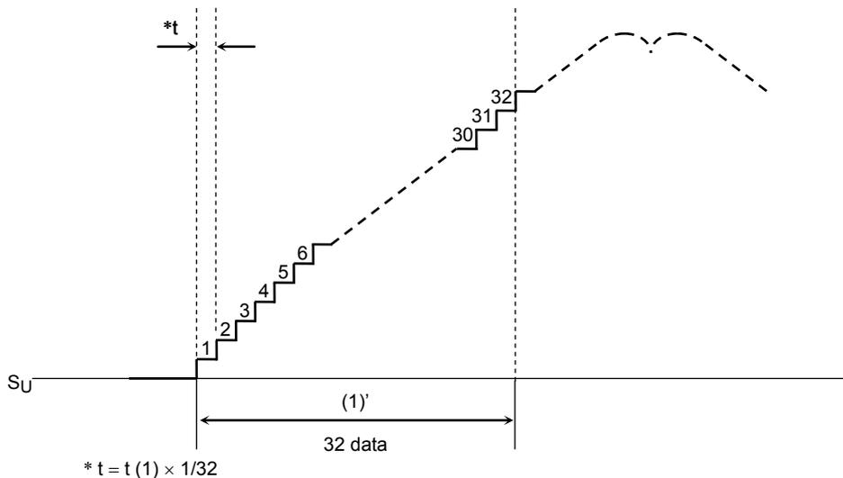
Also, the phase alignment with the modulated waveform is performed at every zero-cross point. The modulated waveform is reset by being synchronized with the rising and falling edges of the position detection signal at every 60 electrical degrees. Therefore, the modulated waveform becomes discontinuous
