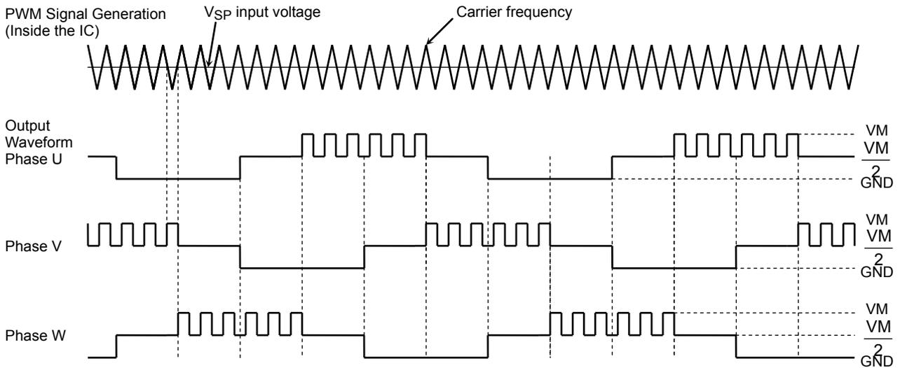
Note: The above U-phase waveform shows the behavior of the U-phase output signal when a resistor is connected between the U and VM pins and also between the U pin and ground to obtain  $\frac{VM}{2}$ . Likewise, resistors are connected to the V and W pins.  $\frac{VM}{2}$  indicates the high-impedance state.
