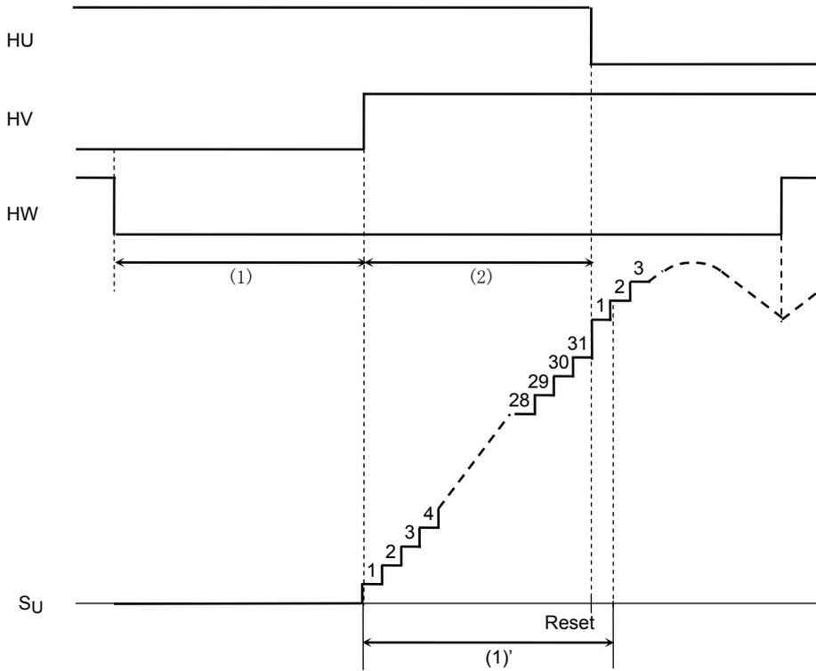
**<Output Waveform of the Sine-Wave PWM Drive>**
