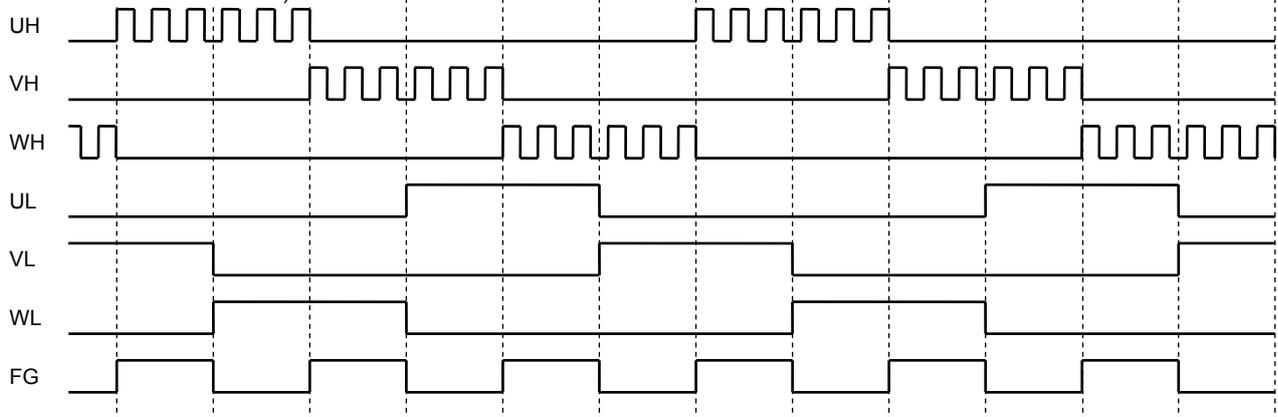
\*: If the Hall signal for clockwise rotation is applied when CW/CCW = High, the motor is driven by the 120° commutation signal with a lead angle of 0°. (Reverse rotation by the wind)
