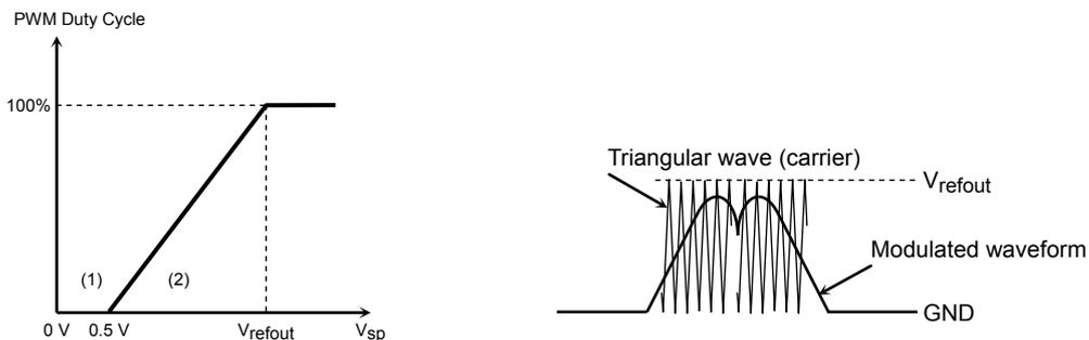
Note: An amplitude of the modulated waveform becomes maximum when  $V_{SP} = V_{refout}$ . The PWM duty cycle that is obtained with the  $V_{SP}$  voltage of  $V_{refout}$  is defined as 100%.
