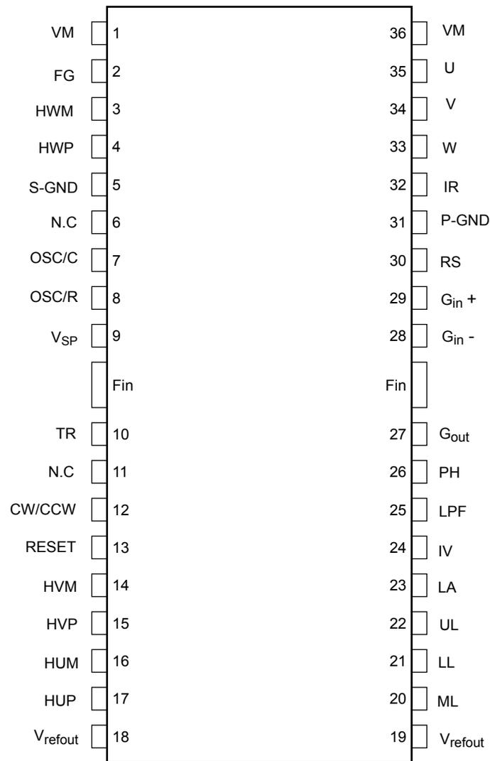
Note: Pins 1 and 36 and pins 18 and 19 are respectively connected together on the frame inside the IC.
