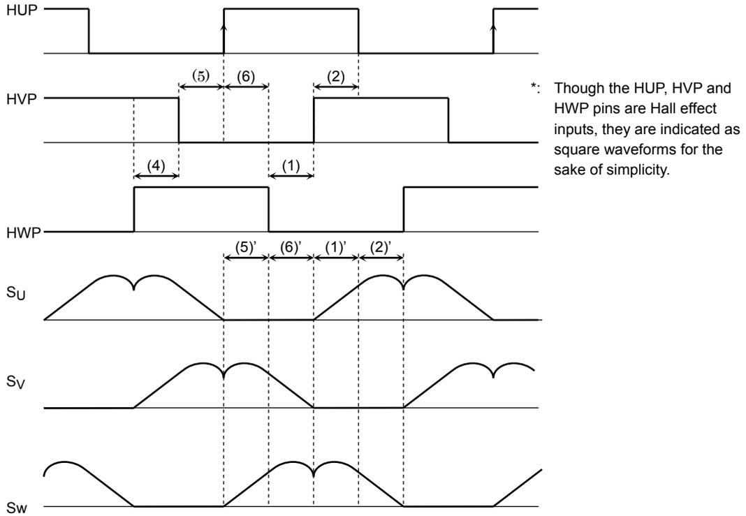
As illustrated above, the modulated waveform (1)' advances by 1/32 of the period between the rising edge (↑) of HU and the falling edge (↓) of HW. Likewise, the modulated waveform (2)' advances by 1/32 of the period between the falling edge (↓) of HW and the rising edge (↑) of HV.
