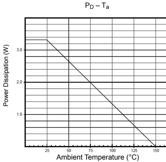
Measured on a board (140 mm × 70 mm × 1.6 mm, Cu: 50%)  $R_{th(j-a)}$  = 38°C/W
