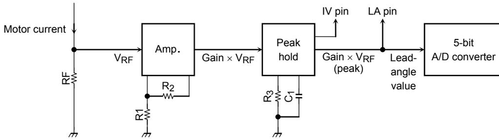
\*: Gain = (R<sub>1</sub> + R<sub>2</sub>) / R<sub>1</sub>, R<sub>3</sub> = 100 kΩ, C<sub>1</sub> = 0.1 μF
