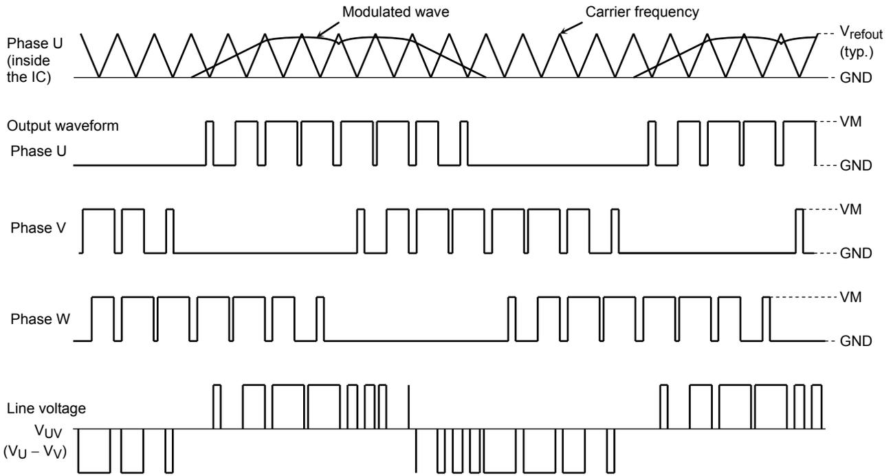
**<Output Waveform of the Square-Wave Drive>**
