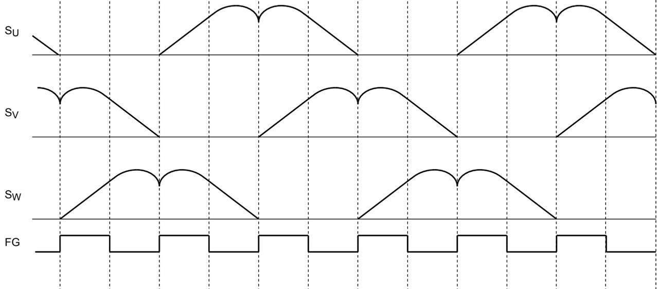
\*: The lead-angle correction is performed in accordance with the LA input when the Hall signal frequency is 2.5 Hz or higher.
