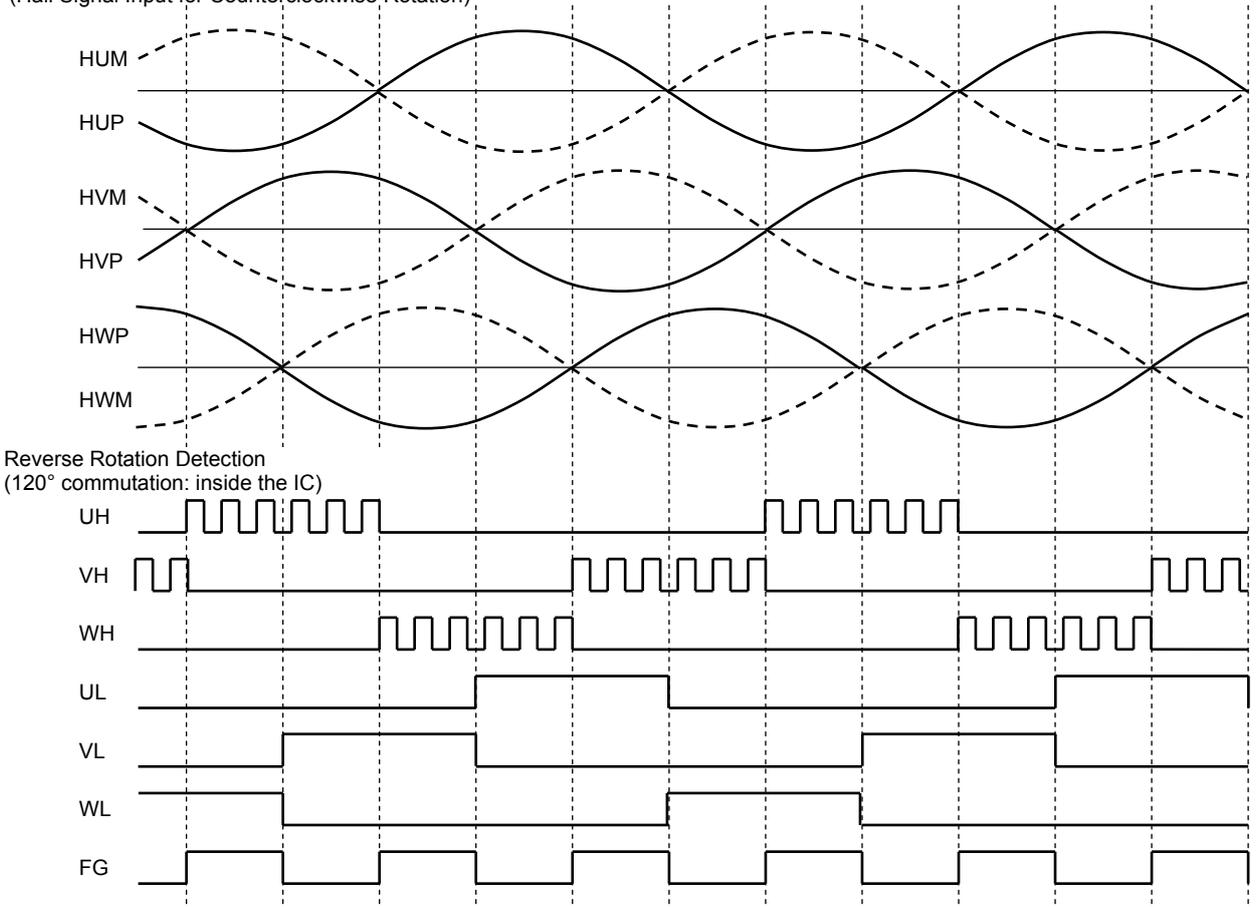
\*: If the Hall signal for counterclockwise rotation is applied when CW/CCW = Low, the motor is driven by the 120° commutation signal with a lead angle of 0°. (Reverse rotation by the wind)
