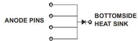
**Note:** All four anode pins must be electrically connected at the printed circuit board.
